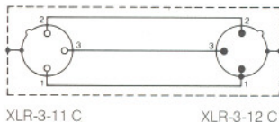
Connecting cable KA 7 U (Art.-No. 1777) Fitted at both ends with XLR-connectors. Length: 7.5 m.
