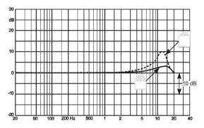
On-axis frequency response of Miniature Microphones. Dotted line is with high boost grid and solid line with soft boost grid.
