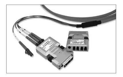
The Extron DVI 104 is a transmitter and receiver set that sends single link DVI signals over long distances up to 500 meters (1,640 feet) over four multimode fiber optic cables. It uses all digital technology to deliver perfect pixel-for-pixel transmission of computer-video images up to 1920x1200 resolution, including HDTV 1080p/60.
