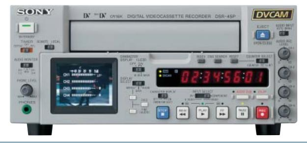
The DSR-45 is best used as a player/recorder in a nonlinear editing suite. When used in A/B roll editing, the DSR-45 can be used as a source feeder. The DSR-45 cannot perform insert or assemble editing nor does it have a synchronization capability.
