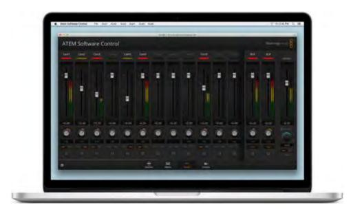
you get complete multi track mixing control with level meters! You can direct camera and external audio with precision level and balance adjustments, enable and disable channels or activate audio follow video mode instantly. You can also connect to Mackie™ standard USB audio mixer panels, giving you hardware feedback and feel of flying faders and meter displays.
