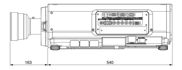
The illustration shows the lens attached to the DLP projector.
