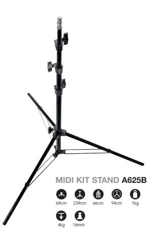
Aluminium stand. 4 sections, 3 risers. Ø: 25, 22, 19, 16mm. Leg Ø: 19mm.
