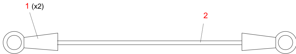
Figure 3-79: Chassis To Yoke Ground Cable Assembly
