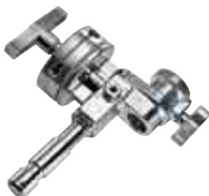
Designed to convert a Junior Stand into an overhead stand, the D400 incorporates a 4-1/2" (10mm) grip head with a junior stud and receiver.
