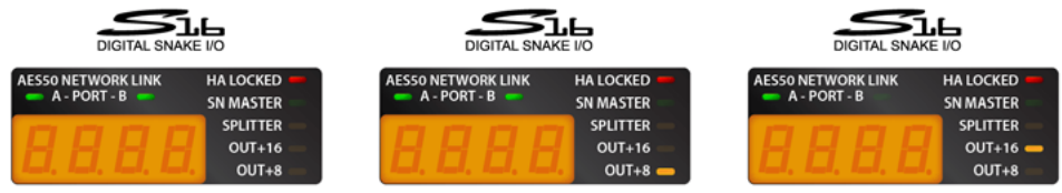
FOH console supplies clock synchronization and controls the S16 preamps exclusively (local HA control is blocked by console)
